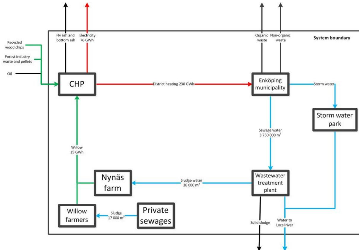
**Picture 1 - Flowchart of the symbiotic system in Enköping. The colors are representing different material types. Blue = Water, Green = Biobased fuels, Red = Energy and Black = Solids. The fly and bottom ash is landfilled, and the non-organic waste is incinerated in Västerås. Organic waste is sent to Uppsala for production of biogas.**
